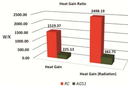
Figure 5-4. Heat Gain in the AGS1 Structure and RC Structure
