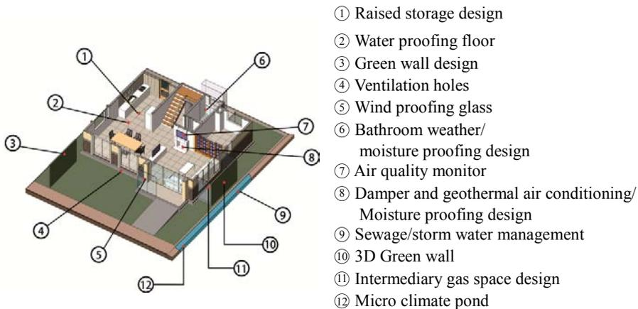
Ground floor Design: Mainly the foundation structure and geothermal air conditioning system, plus the optimal use of space under the floor surface; outdoors are green walls, intermediary gas space, and emergency or auxiliary attachments
