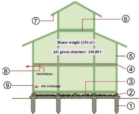
Figure 3-6. Illustration of the Structural System of the AG Innovative Composite Structure
