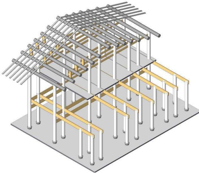
Figure 9. The 3D models of tea house's beams and pillars structure
