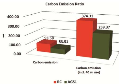
Figure 5-2. Comparison in Carbon emission –the AGS1 Composite vs. RC structures
