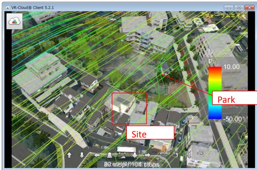
Figure 6 Phase One wind analysis (shown using VR-Cloud).
