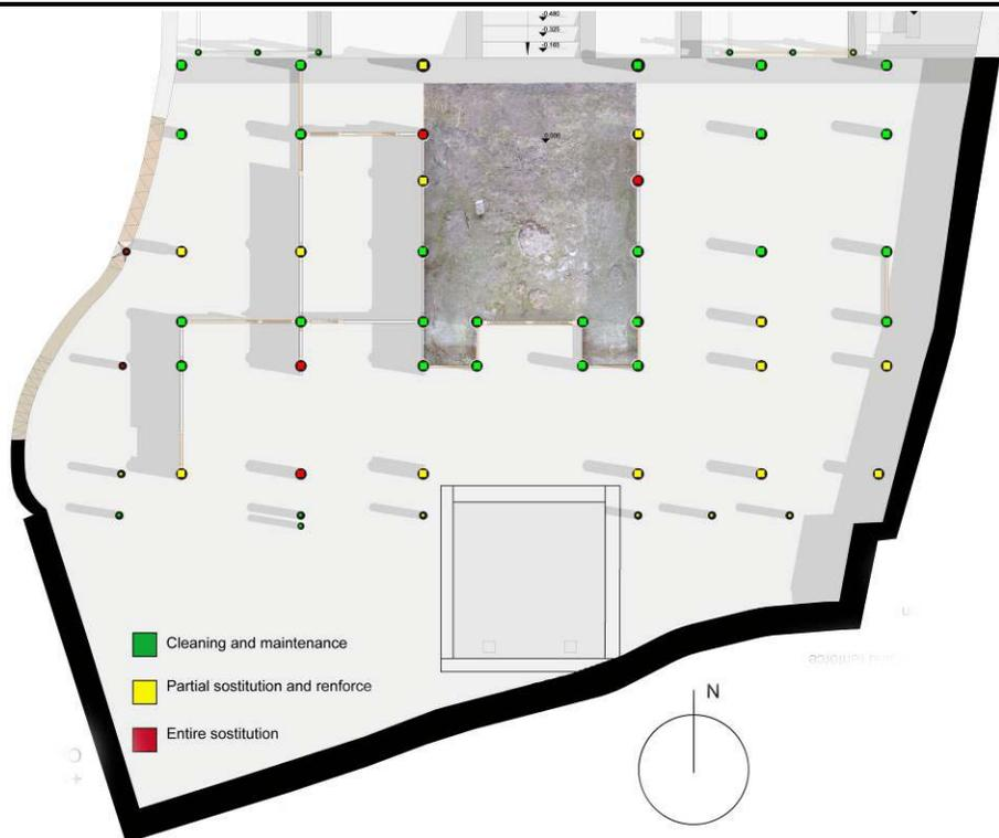
Figure 13. The appropriate disposal measures of the pillars in tea house's 1 floor
