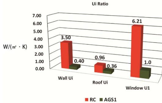
Figure 5-3  $U_i$  Ratio of Each Element between the AGS1 Structure and the RC Structure
