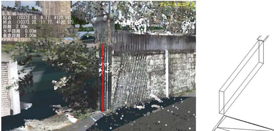
Figure 8 Neighbor building's fence height is reflected into the BIM model
